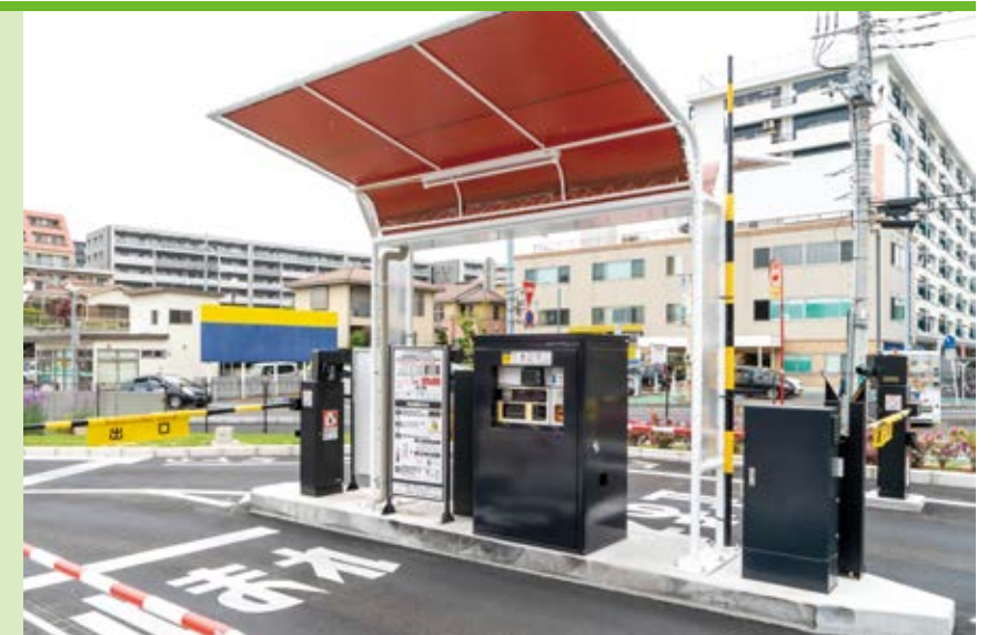
Parking lot management system with plate number recognition
